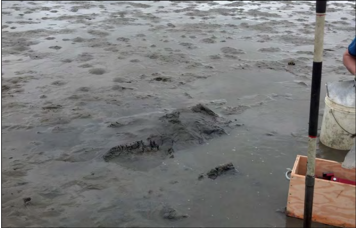
Figure 6: Geologic Probe and test pit #2 showing gray silty sand.
