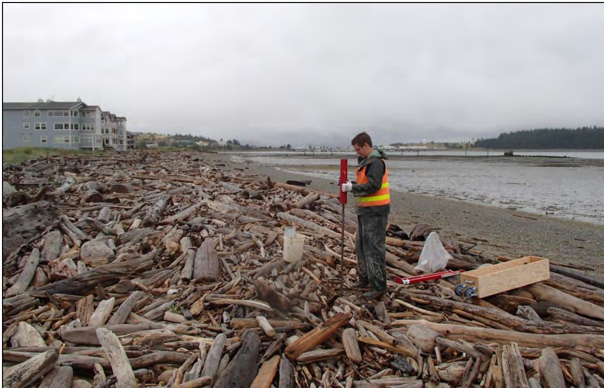
Figure 9: View east, geologic probe being driven in to the ground by hand.
